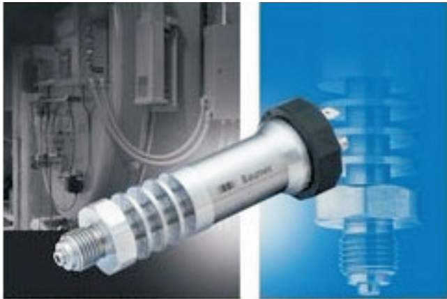
Baumer's PBSN pressure transmitter series can now be used in media temperatures up to 150 °C. This is made possible by means of a cooling neck. Photo: Baumer
